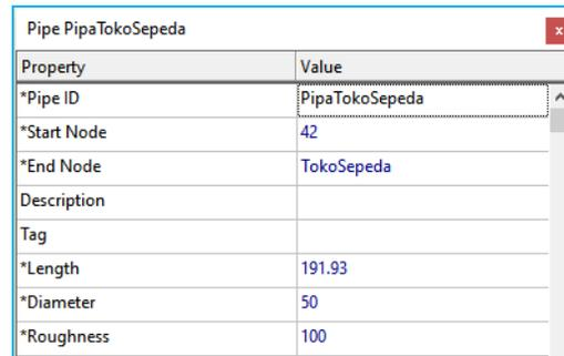
Figure 11. Example of Modified C Value Input in PVC Pipe model 50 mm
