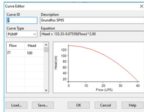
Figure 6. Pump Curve Editor in Epanet
