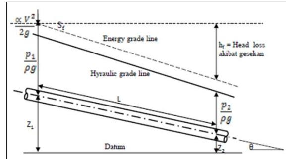
Figure 2. Pressure Line and Energy Line Bernoulli Equation
