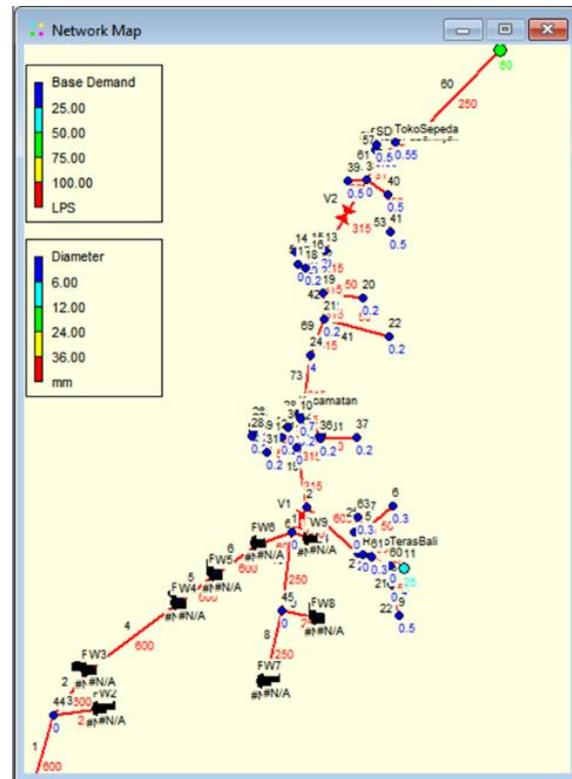
Figure 8. Pump-Pipe Network Model in Kec. Mijen on Epanet
