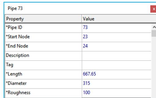
Figure 12. Example of Modified C Value Input in PVC Pipe model 315 mm
