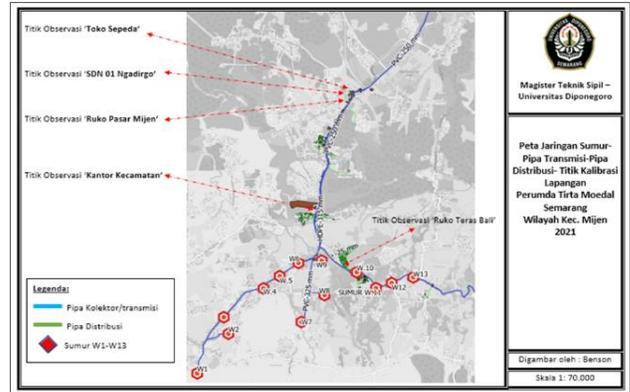
Figure 3. Plot of the Distribution Pump-Pipe Network in Kec. Mijen Semarang City
