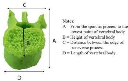
**FIGURE 8.** Accuracy measurement parameter on vertebrae bone
