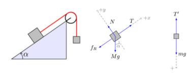
**FIGURE 2**. A block on the ramp and FBD of block
