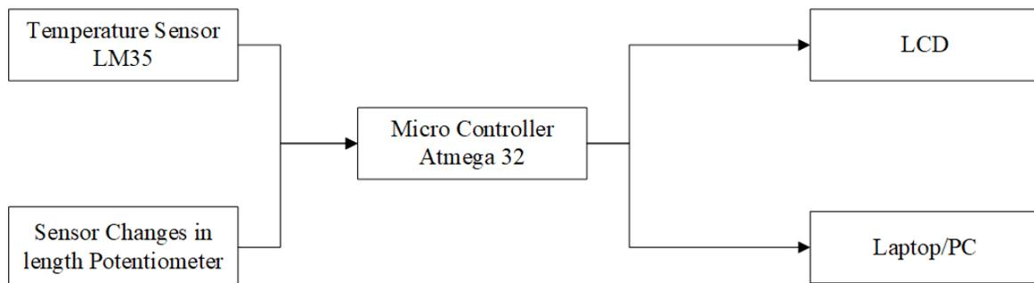
FIGURE 3. Scheme of Thermal Expansion Practicum Sets
