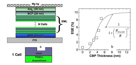
Figure 2 a) The multiple quantum well-like structure used to investigate the concentration quenching mechanism in OLED. b) The plot of external quantum efficiency (EQE) as a function of host thickness shows a good fit with the long-range Förster interaction.
