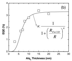
**Figure 3** EQE versus  $Alq_3$  thickness (squares) and the fitting curve (solid line) utilizing the Förster-type quenching rate, with  $R_{Fnr2D} = 6.5$  nm.
