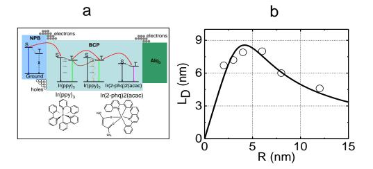
**Figure 4.** a) Illustration of organic light-emitting diode (OLED) structure utilized to measure the exciton diffusion length  $(L_D)$  of  $Ir(ppy)_3$  as a function of intermolecular-spacing. b) The measured  $L_D$  as a function of intermolecular-spacing.
