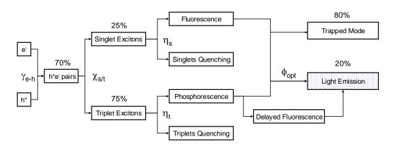
Figure 1 Electroluminescence diagram in OLED
