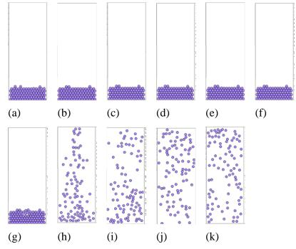
**FIGURE 3.** Particle motion in simulation of fluidization process using gas fluid with fluid velocity increase: (a) 0 m/s, (b) 10 m/s, (c) 20 m/s, (d) 30 m/s, (e) 40 m/s, (f) 50 m/s, (g) 60 m/s, (h) 70 m/s, (i) 80 m/s, (j) 90 m/s, and (k) 100 m/s.
