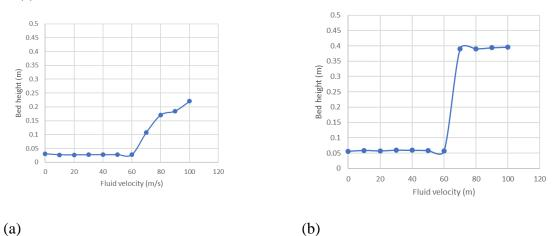
FIGURE 4. Average and maximum bed height in a simulation of the fluidization process using gas fluid.
