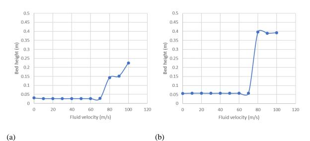
FIGURE 6. Average and maximum bed height in a simulation of the fluidization process using liquid fluid.
