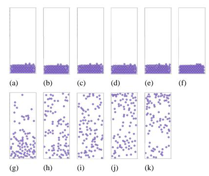
**FIGURE 5.** Particle motion in a simulation of fluidization process using liquid fluid with fluid velocity increase: (a) 0 m/s, (b) 10 m/s, (c) 20 m/s, (d) 30 m/s, (e) 40 m/s, (f) 50 m/s, (g) 60 m/s, (h) 70 m/s, (i) 80 m/s, (j) 90 m/s, and (k) 100 m/s.
