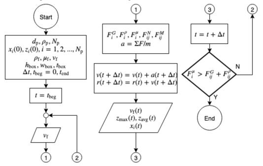
FIGURE 1. Flowchart diagram of simulation of the fluidization process in a two-dimensional vertical box.
