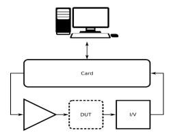
FIGURE 3. Block diagram of characterization system.
