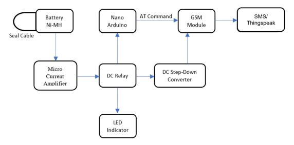
FIGURE 1. Electronic Seal Principles Block Diagram
