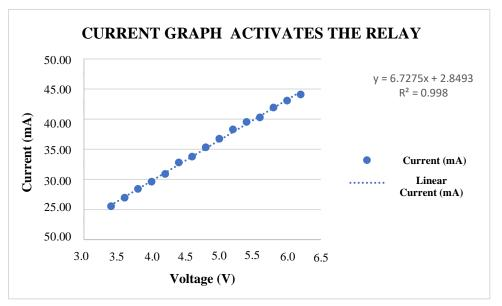
FIGURE 3. Regression Data for Relay Voltage and Current Measurement
