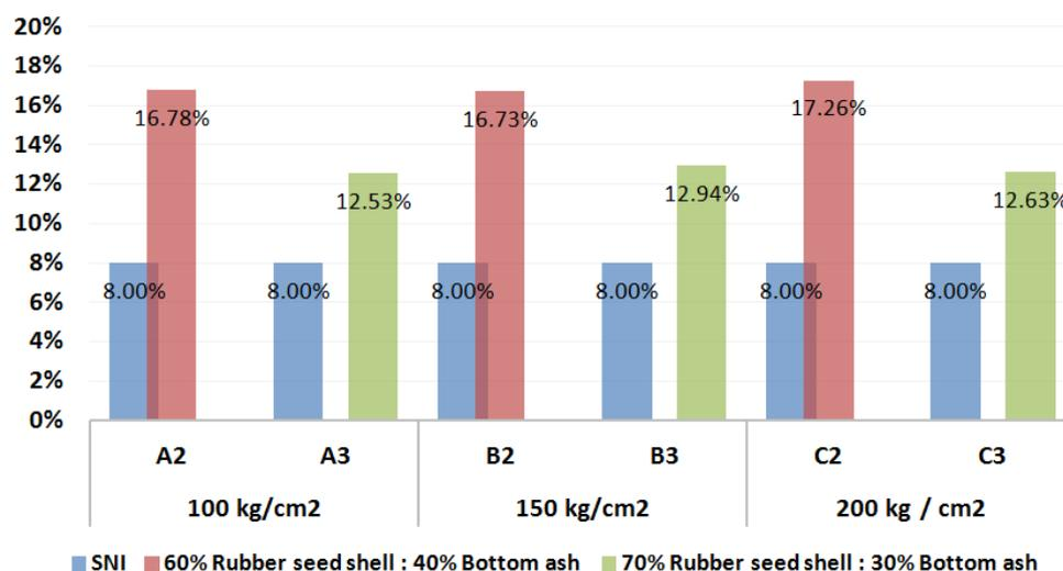
FIGURE 3. The ash content of rubber seed shell and coal bottom ash briquettes.
