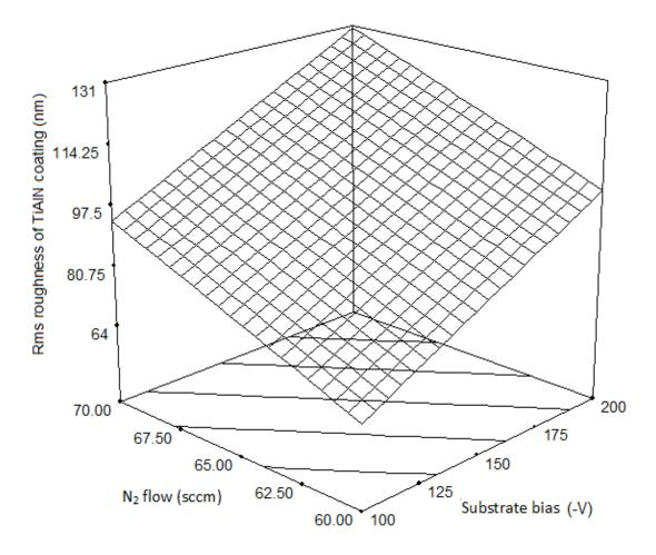
**FIGURE 3.** Three dimension graph of RMS roughness of sputtered TiAlN coatings as a function of negative substrate bias and nitrogen flow rate fall.
