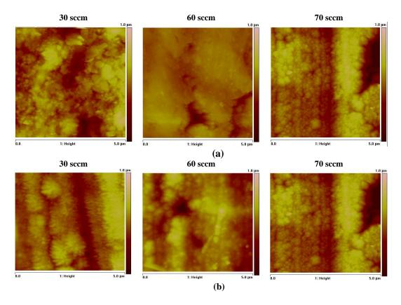
FIGURE 2. The surface morphology of sputtered TiAlN coatings at substrate bias of (a) -100 Volt (b) -200 Volt.
