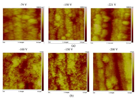
**FIGURE 1.** The surface morphology of sputtered TiAlN coatings at snitrogen flow rate of (a) 65 sccm (b) 30 sccm.
