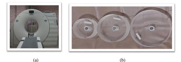
**FIGURER 2.** Research Tools. (a) CT Scan Siemens Somaton Emotions 16, (b) solid water phantom pf various diameters.
