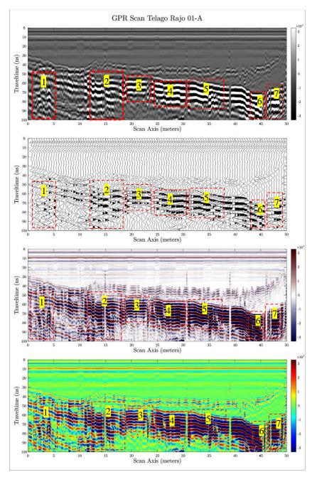
FIGURE 10. GPR Imaging Telago Rajo; (a) Grayscale view; (b) Wiggle view; (c) Blue-Red view; (d) Jet view.
