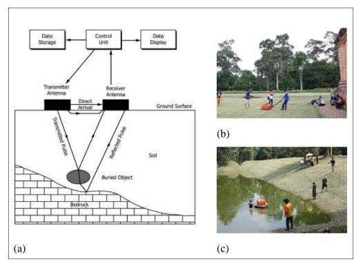
**FIGURE 4**. (a) Basic Principal of GPR [11]; (b) GPR acquisition at Gumpung Temple; (c) GPR acquisition at Telago Rajo.
