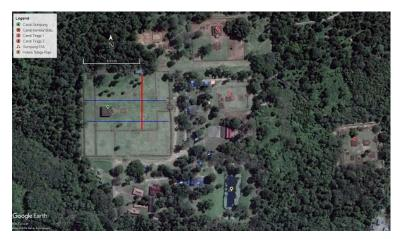
**FIGURE 6.** Location of GPR data acquisition; Gumpung Temple show with green balloon symbol. Two parallel blue lines West-East direction on Gumpung are Line 01-A and Line 02. Telago Rajo Pool show with yellow balloon symbol. Blueline at Telaga Rajo Pool is Line 04.
