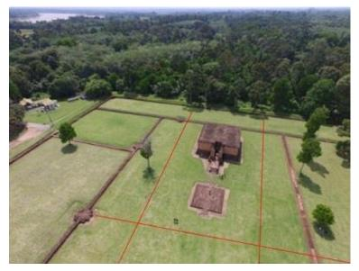
FIGURE 5. Image of Gumpung Temple using UAV (drone). Red line shows our GPR scans.
