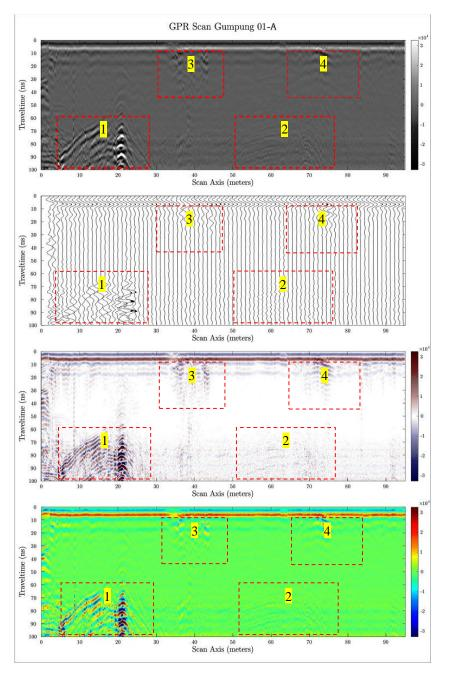
FIGURE 7. GPR Imaging Gumpung 01-A; (a) Grayscale view; (b) Wiggle view; (c) Blue-Red view; (d) Jet view.
