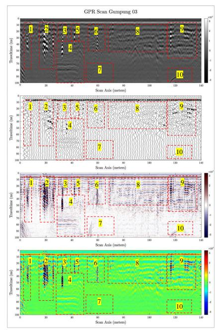
FIGURE 9. GPR Imaging Gumpung 03; (a) Grayscale view; (b) Wiggle view; (c) Blue-Red view; (d) Jet view.
