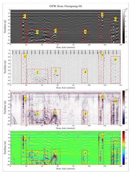
**FIGURE 8**. GPR Imaging Result Gumpung 02; (a) Grayscale view; (b) Wiggle view; (c) Blue-Red view; (d) Jet view.
