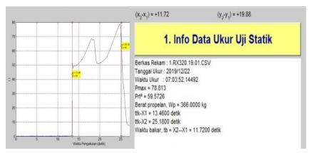
FIGURE 5. Numerical Data Acquisition Result of Combustion Chamber Pressure from Static Test of RX320.
