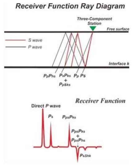
FIGURE 3. The simple wave propagation diagram to identificating conversion phase of P wave [9].
