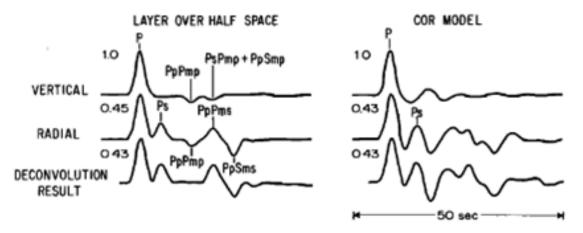
FIGURE 2. Deconvolution tecnic using two planes earth's layer (Langston, 1979)
