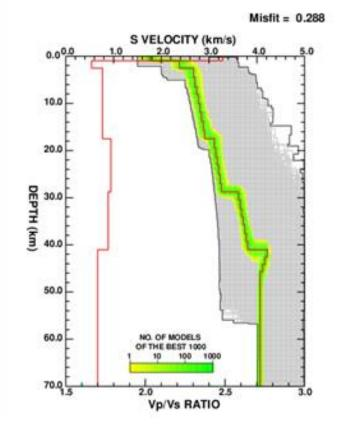
FIGURE 6. The S wave velocity profile and Vp/Vs ratio under LBFI station.
