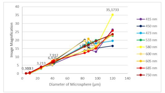
**FIGURE 2.** Image magnification as a function of microsphere's diameter for each light-source in visible light spectrum using barium titanate microsphere in free-space. The largest magnification is yielded when the light-source has a wavelength of 580 nm (yellow).
