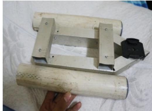
**Gambar 7.** Body Robot ROV
