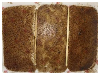
(A) (B) (C) Gambar 4 Bioplastik (A) 5 gram pati kulit pisang + 10 gram pati ubi jalar (B) 5 gram pati kulit pisang + 5 gram pati ubi jalar (C) 10 gram pati kulit pisang + 5 gram pati ubi jalar (Sumber : Penulis)
