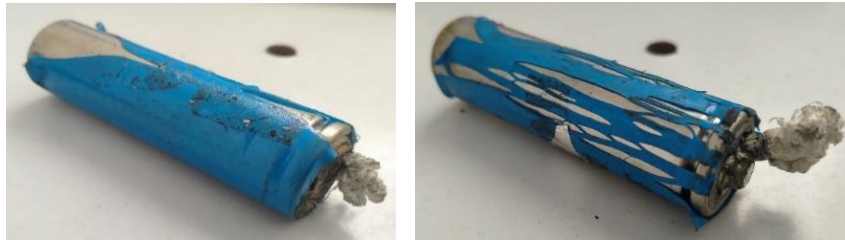
Figure 19. Physical condition of the battery after explosion at 50% state of charge, Test 1 (a) and Test 2 (b)
