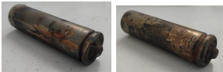
Figure 15. Physical condition of the battery after explosion at 0% state of charge, Test 1 (a) and Test 2 (b)
