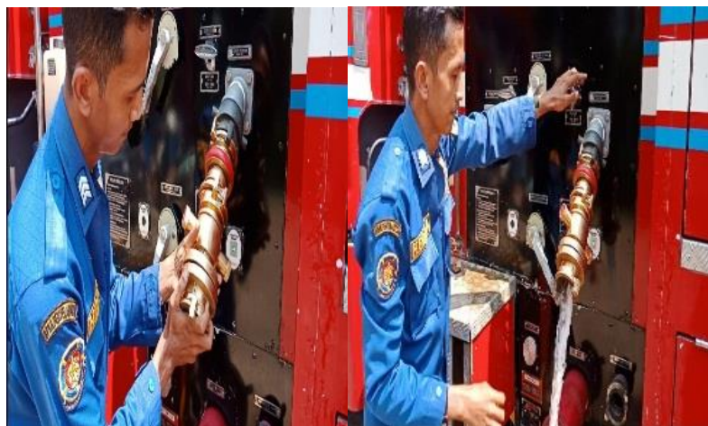
Figure 2. Leak Testing Adaptor Coupling.
