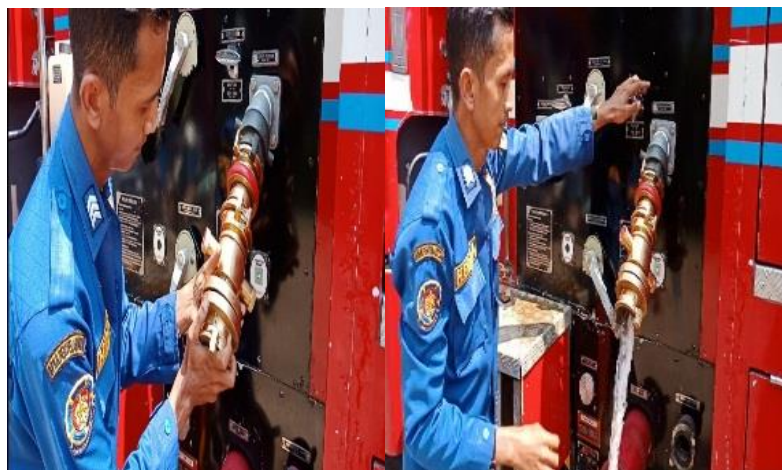
Figure 2. Leak Testing Adaptor Coupling .
