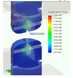
Fig.9 Stress distribution on the grip for copper (Cu)
