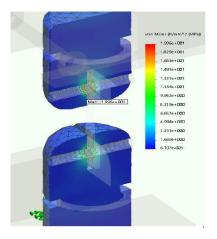
Fig.8 Stress distribution on the grip for Al 6061
