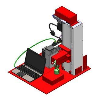
Fig. 2 Tensile testing machine model
