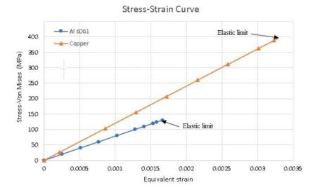
Fig. 9 Stess - strain curve for aluminium 6061 and copper
