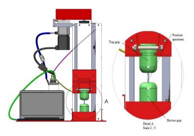
Fig. 3 Position of the specimen
