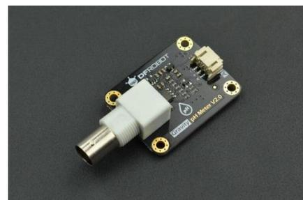
**Gambar 2.3** Transmitter SEN0161 V2
