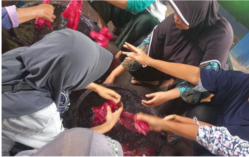
Figure 4. The dyeing process of batik fabric is carried out after the waxing
