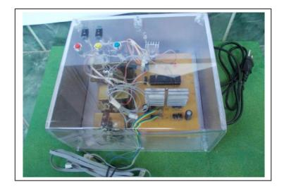
3. Trial Model of the Miniature Magnetic Levitation Train
