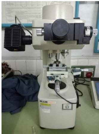
**Gambar 6.** Mesin Uji Keras HM-122
