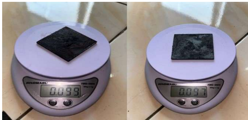
Figure 7. Specimen weighing process after immersion
