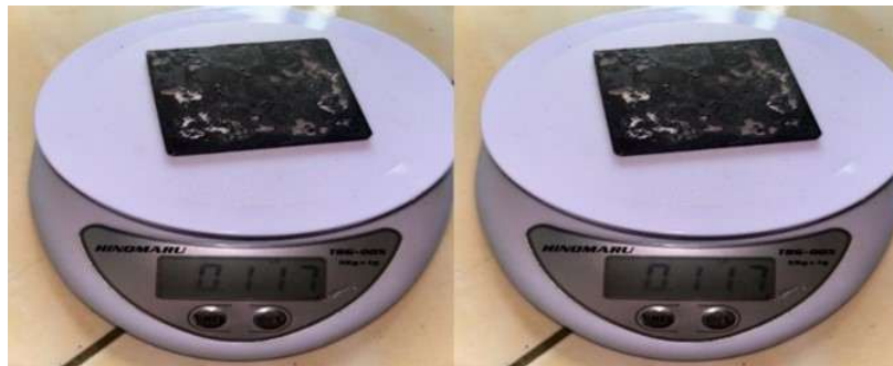
Figure 6. Specimen weighing process before immersion
