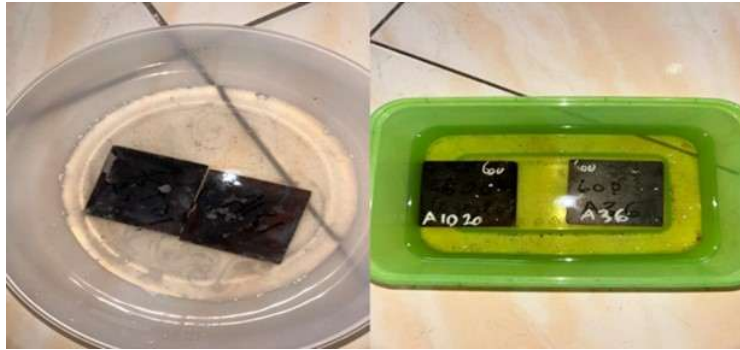
Figure 5. Sulfuric acid soaking process
