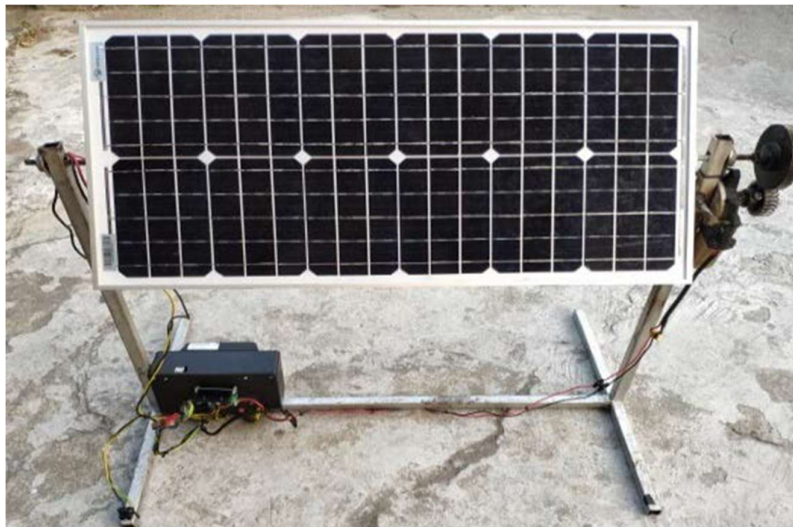
Figure 4. PV panel with solar tracker single-axis [11]
