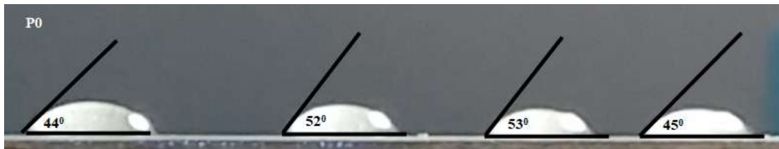
Figure 12. Contact angle of PU samples
