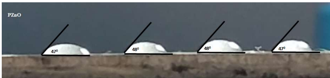
Figure 14. Contact angle of PZnO samples
