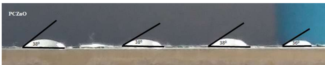
Figure 15. Contact angle of PCZnO samples
