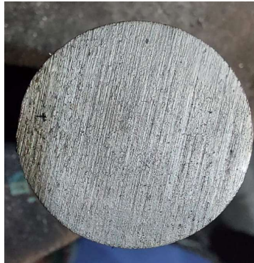
Figure 11. Non-heat treatment specimen specimens for Brinell hardness test
