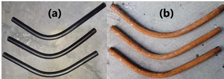
Figure 8. Bending results–single quenching specimens using (a) Oil and (b) Air as quenching media
