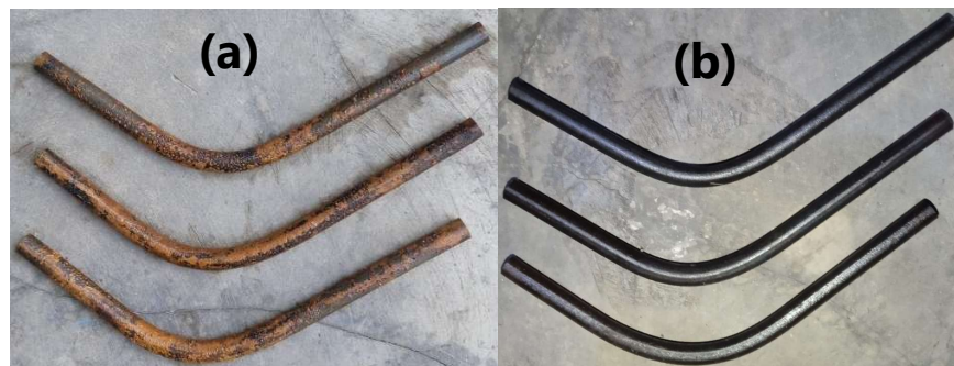
Figure 9. Bending test results of double quenched specimens (a) Oil–air and (b) Oil–oil as quenching media
