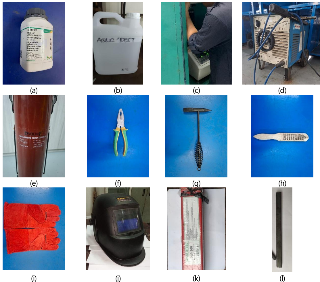
Figure 1. Tools and materials (a) Sodium chloride, (b) Distilled water, (c) Vickers hardness, (d) Welding machine, (e) Electrode oven, (f) pliers, (g) chipping hammer, (h) Wire brush, (i) Welding gloves, (j) Welding helmet, (k) electrode, and (l) Carbon steel
