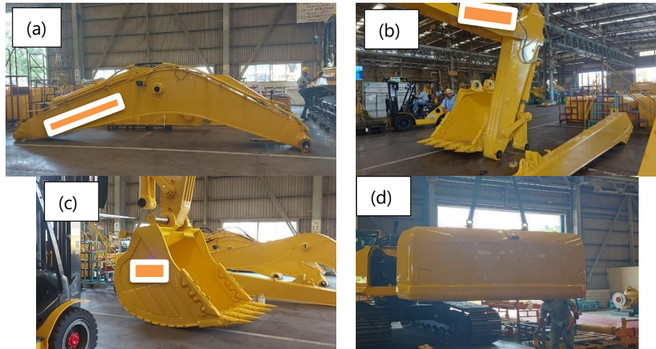
Figure 3. Excavator parts (a) Boom, (b) Arm, (c) Bucket, and (d) Counterweight
