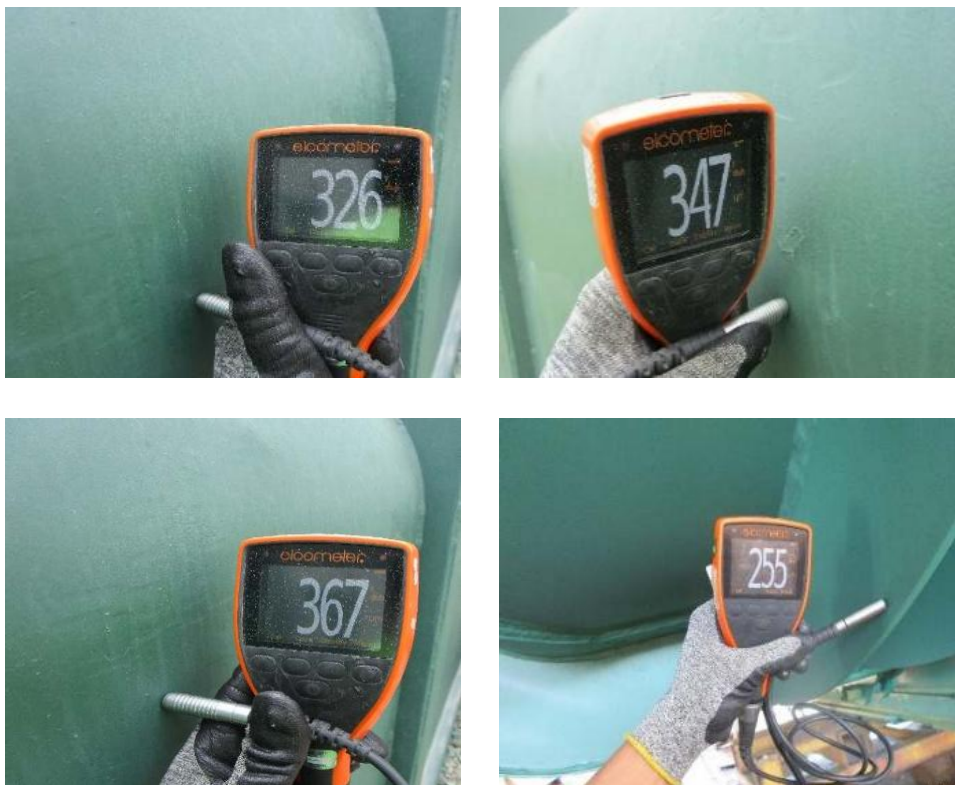
Figure 5. Primer coat thickness
