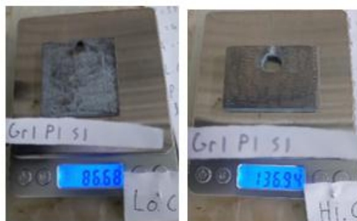
Figure 4. Specimen conditions after the coating process (Left: AISI 1020; Right: AISI 1070)
