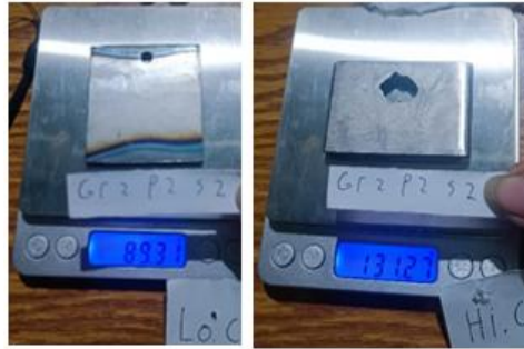
Figure 7. Specimen conditions after the pickling process (Left: AISI 1020; Right: AISI 1070)
