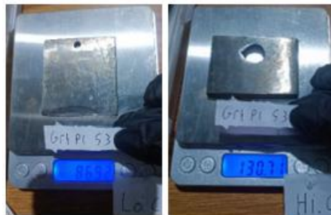
Figure 5. Specimen conditions after the pickling process (Left: AISI 1020; Right: AISI 1070)
