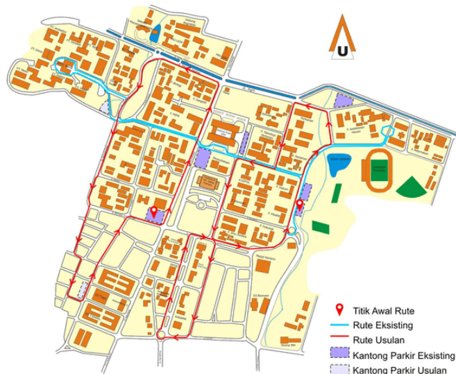
Gambar 12. Layout Usulan Perancangan Bus Kampus
