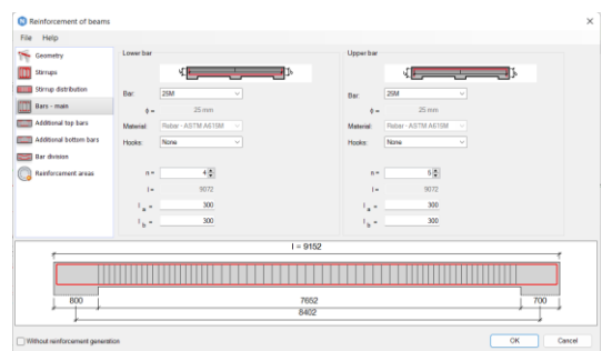
Figure 4. Main rebar data entry
