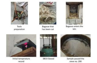
Figure 2. Sample preparation process
