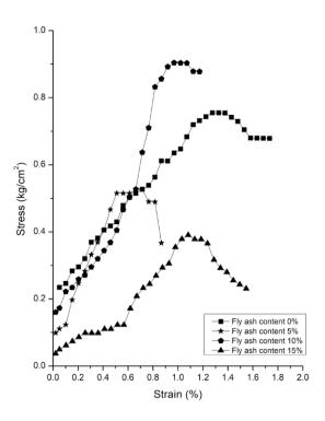
Figure 3. Stress-strain relationship obtained from UCT
