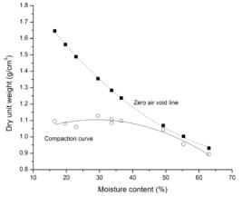
Figure 2. Compaction curve and zero air void line
