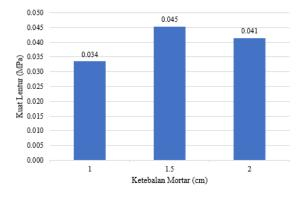
Figure 8. Flexural test averages
