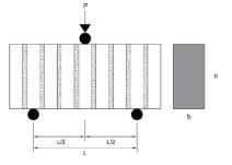
Figure 2. Flexural test (SNI 4154, 2014)
