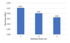
Figure 7. Direct shear test averages
