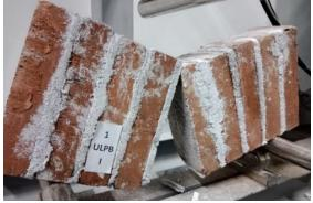
Figure 12. Failure pattern 1 ULPB
