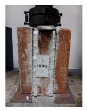
Figure 9. Failure pattern of 1 UGPB
