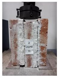
Figure 11. Failure pattern of 2 UGPB
