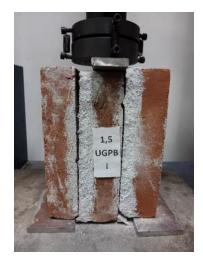
Figure 10. Failure pattern of 1.5 UGPB
