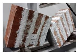
Figure 13. Failure pattern 1.5 ULPB
