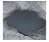
Figure 2. Admixture Silica Fume
