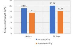
Figure 4. Compressive Strength of Normal Concrete
