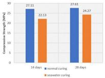
Figure 7. Compressive Strength of 6% B + 20% SF Concrete
