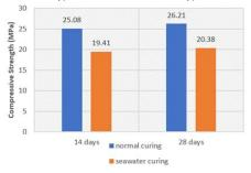
Figure 5. Compressive Strength of 6% B + 0% SF Concrete
