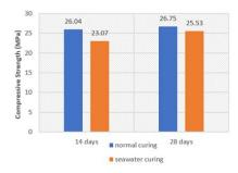
Figure 8. Compressive Strength of 6% B + 25% SF Concrete
