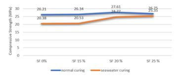
Figure 10. Declining Concrete Compression Test During Seawater During 28 Days
