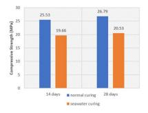
Figure 6. Compressive Strength of 6% B + 15% SF Concrete
