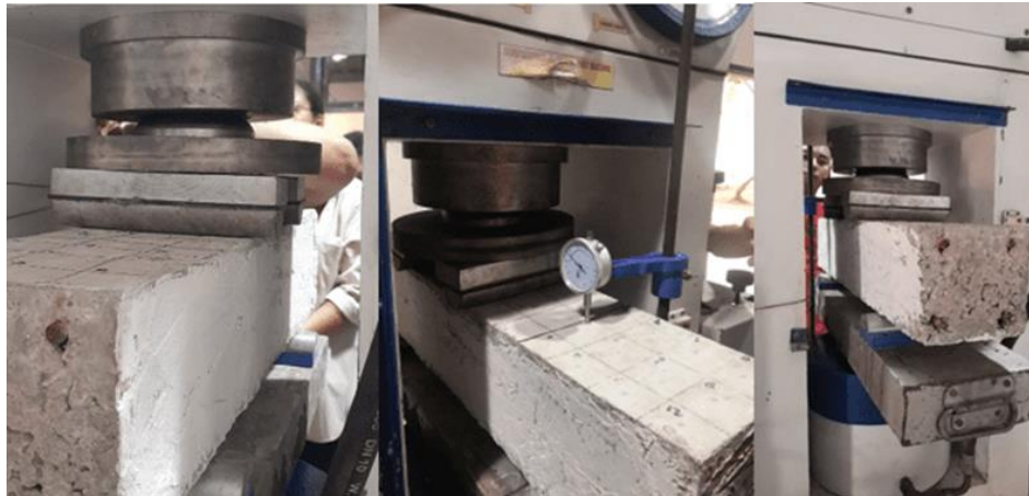
Figure 10. Reinforced concrete beam testing
