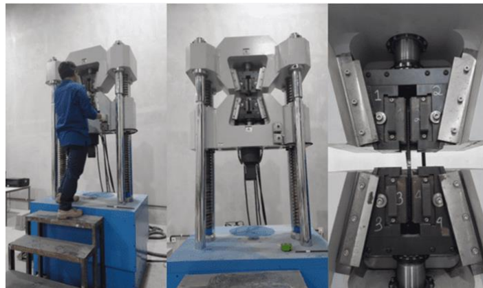
Figure 8. The process of preparing the tensile test of D-10 reinforcement
