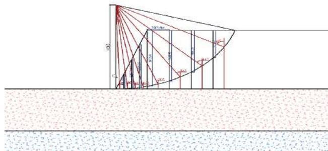
Figure 2. Original Slope Analysis of Embankment Soil Using the Fellenius Method Without Reinforcement
