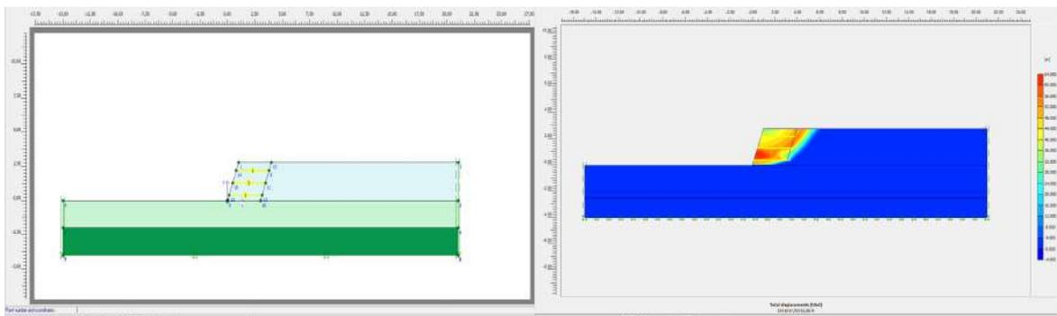
Figure 6. Geometry and Total Displacement of Embankment Slope with MSE Geosynthetic Reinforcement in Plaxis Application.
