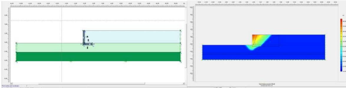
Figure 5. Geometry and Overall Displacement of the Embankment Slope with Cantilever Retaining Wall Reinforcement in the Plaxis Application
