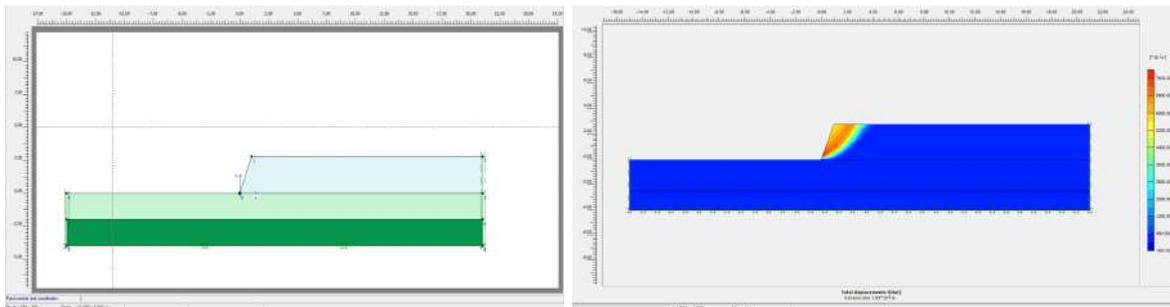
Figure 4. Geometry and Total Displacement of the Fill Soil Slope Without Reinforcement in Plaxis Application.
