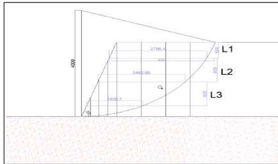
Figure 3. Geometric Layout of Embankment Soil with MSE Geosynthetic Reinforcement.
