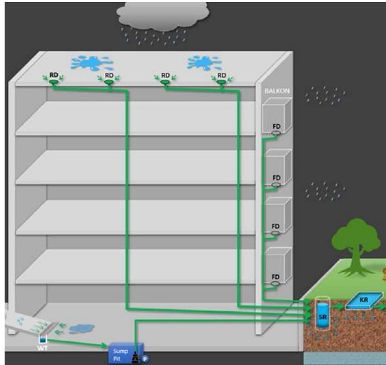
Figure 5. Rainwater Harvesting System on a Regional Scale (Industri)
