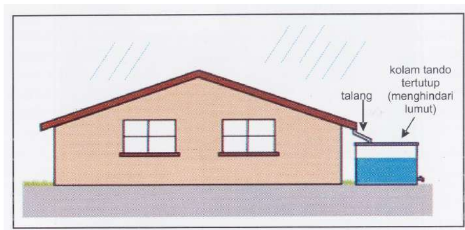
Figure 4. Rainwater Harvesting System on a Parcel Scale
