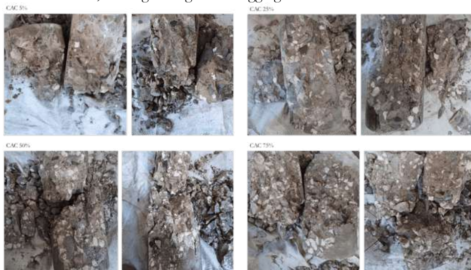
Figure 11. Distribution of coral aggregate particles on cylindrical specimens of CAC
