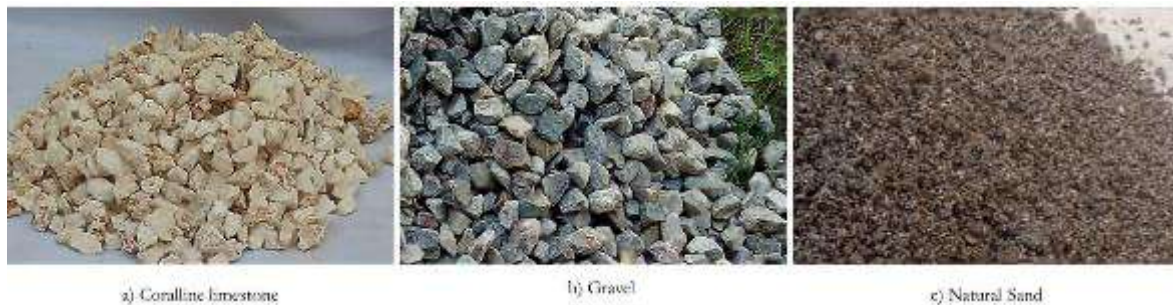
Figure 2. Concrete forming aggregate
