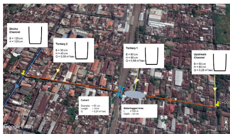
Figure 1. Drainage System in Sriwijaya
