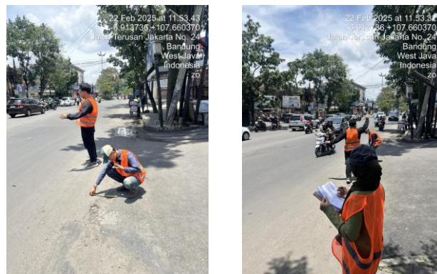
Figure 2. Manual Road Condition Survey
