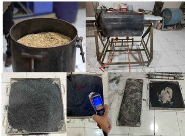
Figure 4. The Process of Burning and Cooling Rice Husks at UKI Civil Engineering Laboratory Reaches 600 °C
