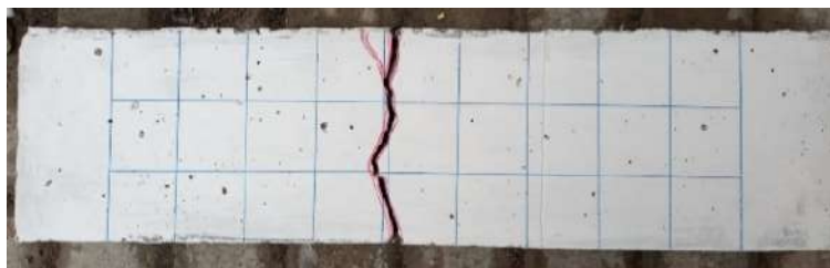
Figure 7. Crack and fracture patterns Sample 15% turnout variation
