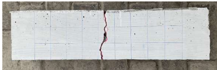
Figure 6. Crack and fracture patterns Sample 10% turnout variation
