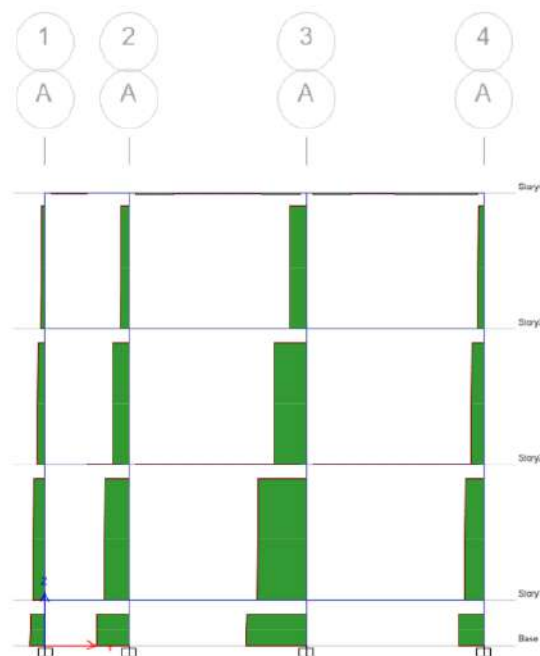
Figure 11. Axial Force ETABS
