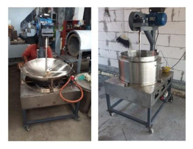
Figure 2. The temperature-controlled shrimp paste mixer machine
