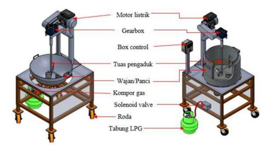
Figure 1. The design of the shrimp paste mixer machine
