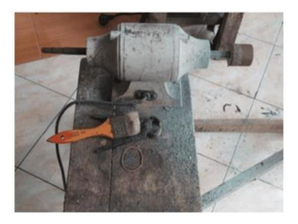
**Figure 2.** Slipper machine without safety and without vacuum cleaner
